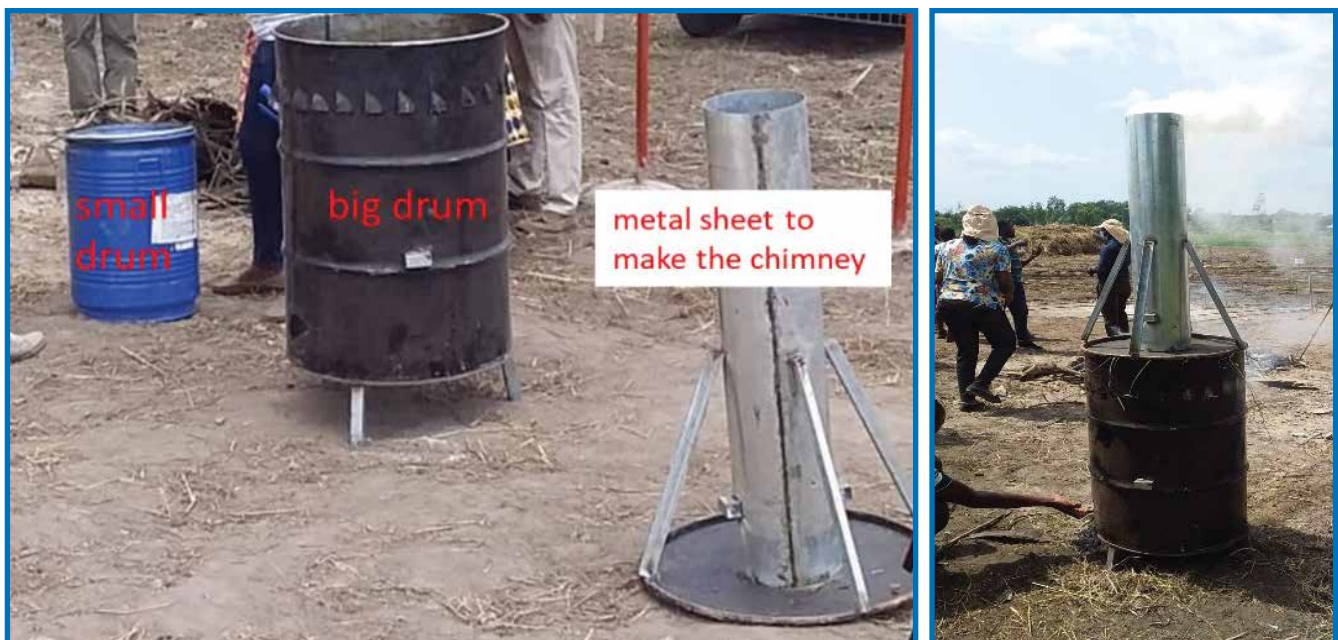
Photo 1. Materials needed to set up the biochar unit.
